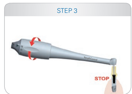
The screw automatically stops when the selected torque is reached
